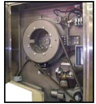
**Mechanical Tilt Mechanism Side**
